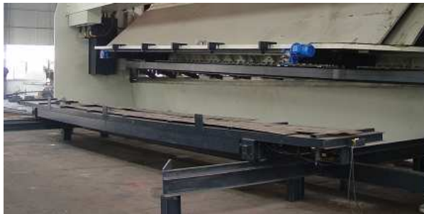
Motorized blade clearance adjusting system, be adjusted through operating the PLC, convenience to adjust the blade gap according the different sheet thickness.
